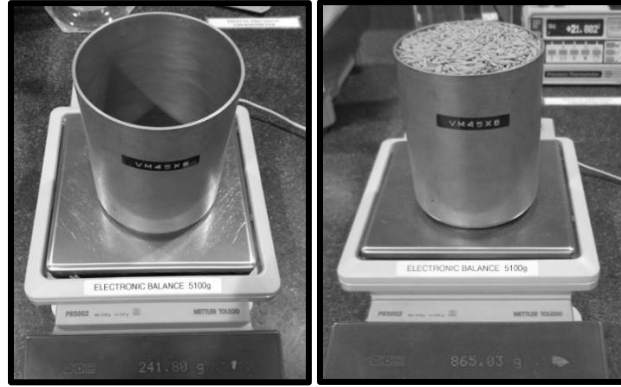
Figure 2. Paddy Density Estimation Using 1 L Density Cup
